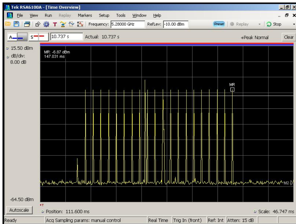
Figure 5-1. Type 1 Radar Pulse
