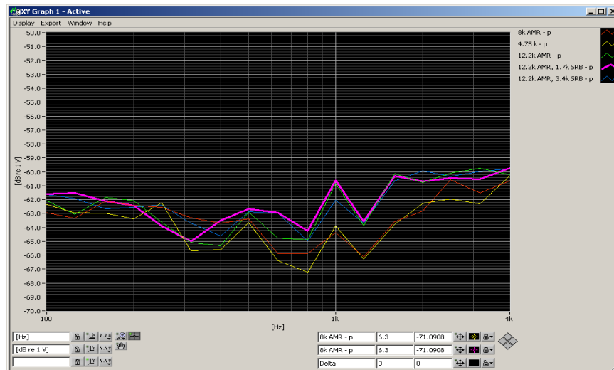
Figure 5-2 UMTS Audio Band Magnetic Noise
