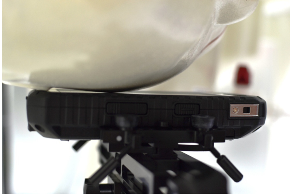
SAR Test Setup Photo 1: Right Cheek
