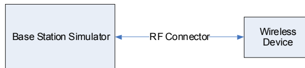
Figure 9-2 Power Measurement Setup
