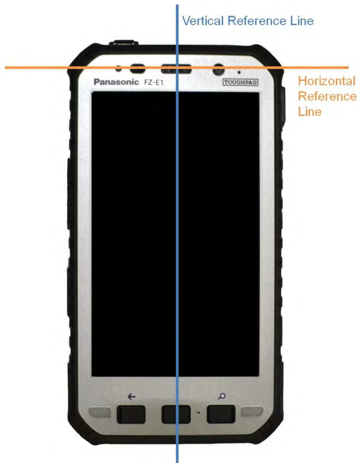
SAR Test Setup Photo 18: Horizontal and Vertical Reference Lines
