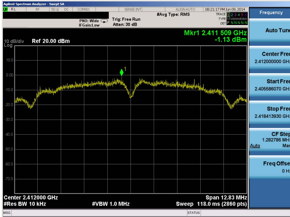
Plot 6-10. Power Spectral Density Plot (802.11b – Ch. 1)
