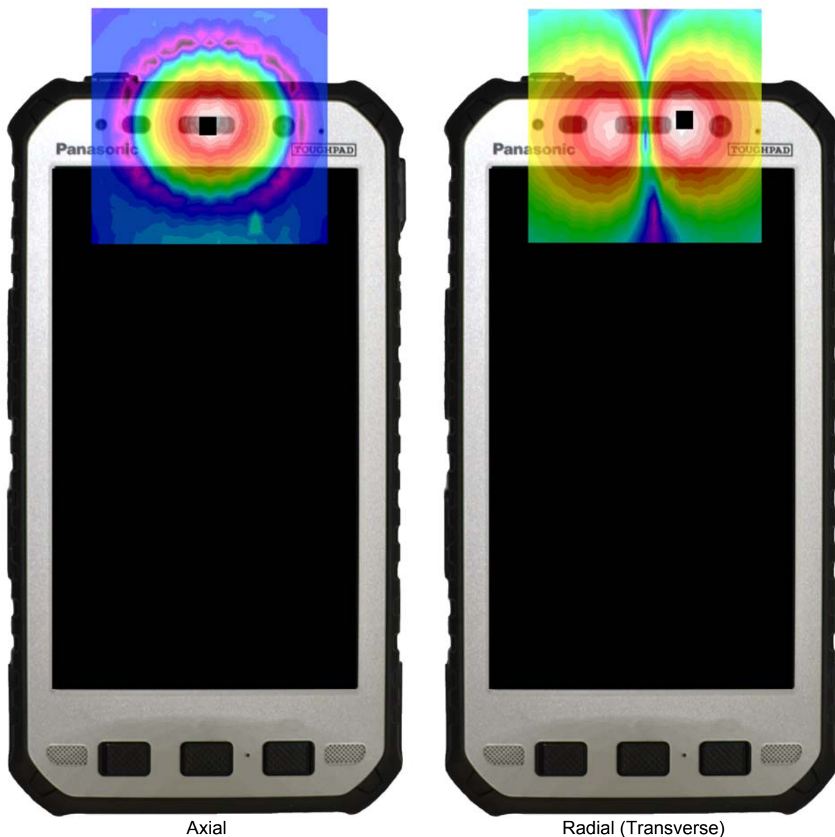
Figure 14-3 T-Coil Scan Overlay Magnetic Field Distributions
