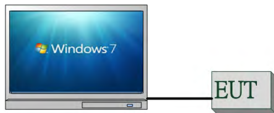
Fig.2-3 Conducted Emission (AC power line) Configuration
