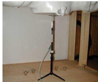
Figure 9-2 System Verification Setup Photo
