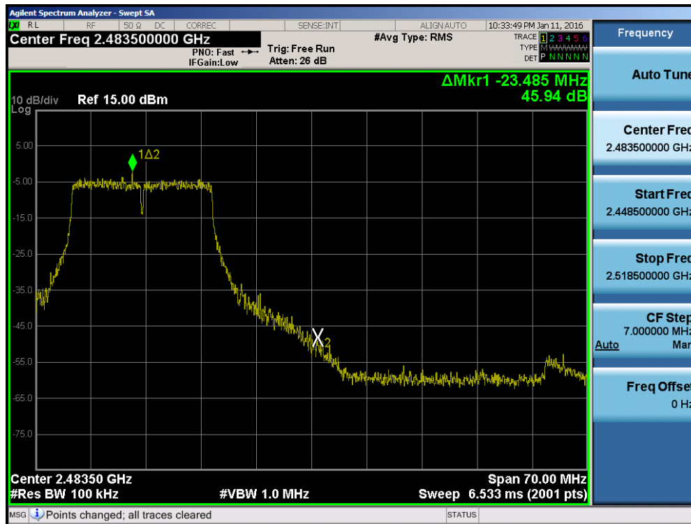
Plot 7-30. Band Edge Plot (802.11n (2.4GHz) – Ch. 11)
