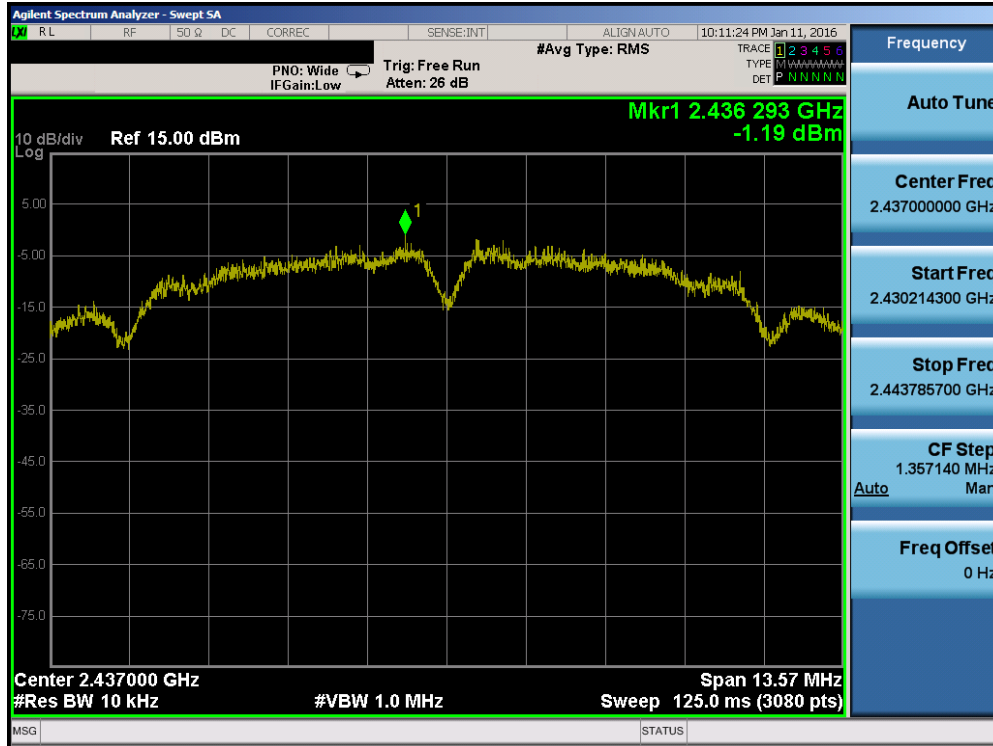
Plot 7-11. Power Spectral Density Plot (802.11b – Ch. 6)
