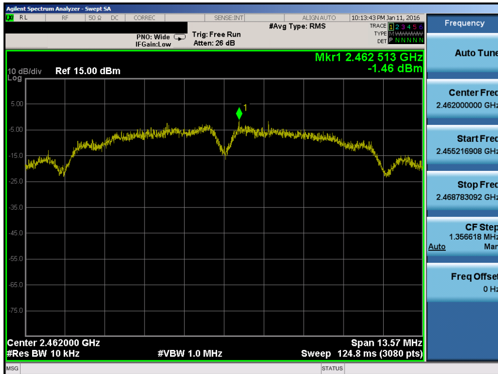
Plot 7-12. Power Spectral Density Plot (802.11b – Ch. 11)
