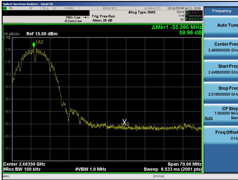
Plot 7-21. Band Edge Plot (802.11b – Ch. 10)
