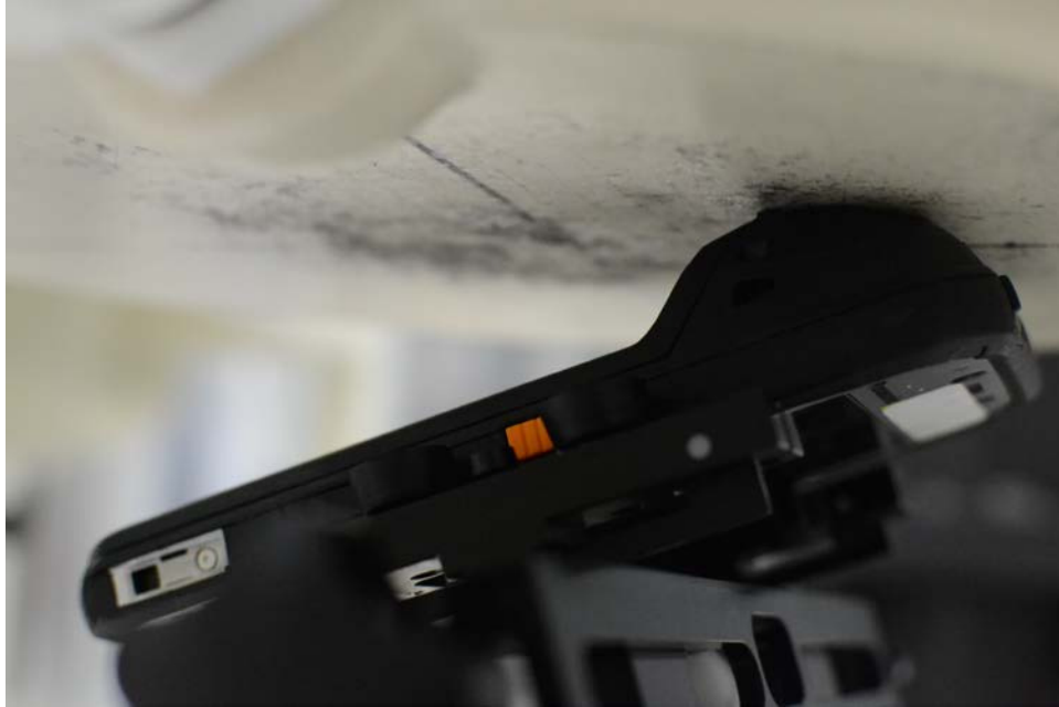
SAR Test Setup Photo 9: Back Side (Tilt) at 0.0 cm with Standard Battery
