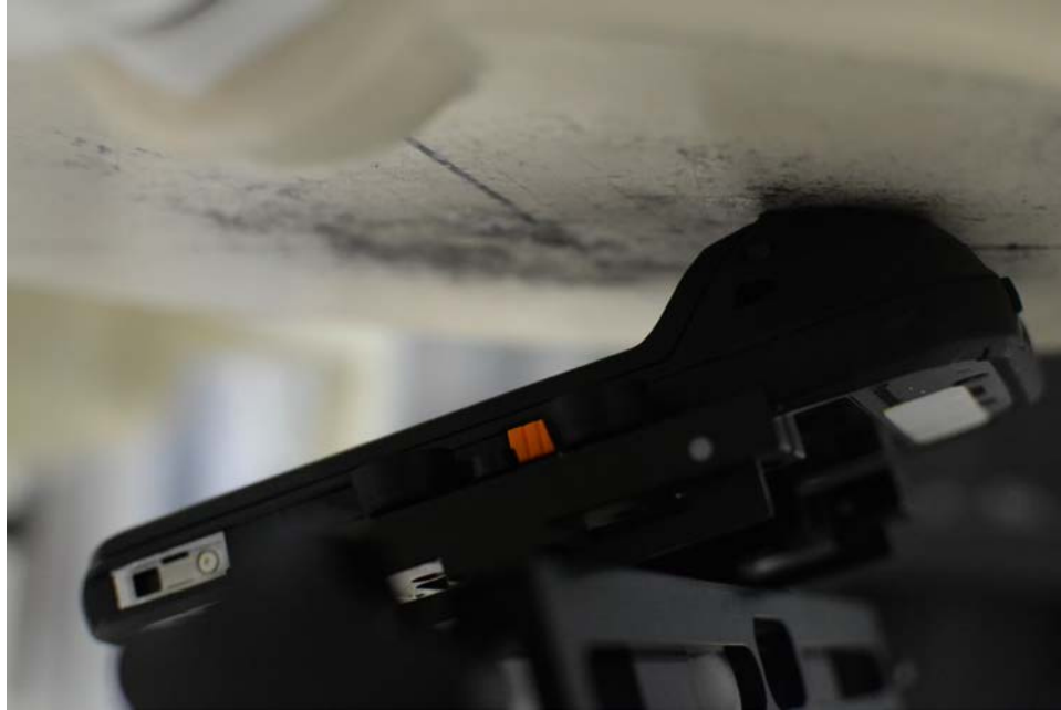
SAR Test Setup Photo 7: Back Side (Tilt) at 0.0 cm
