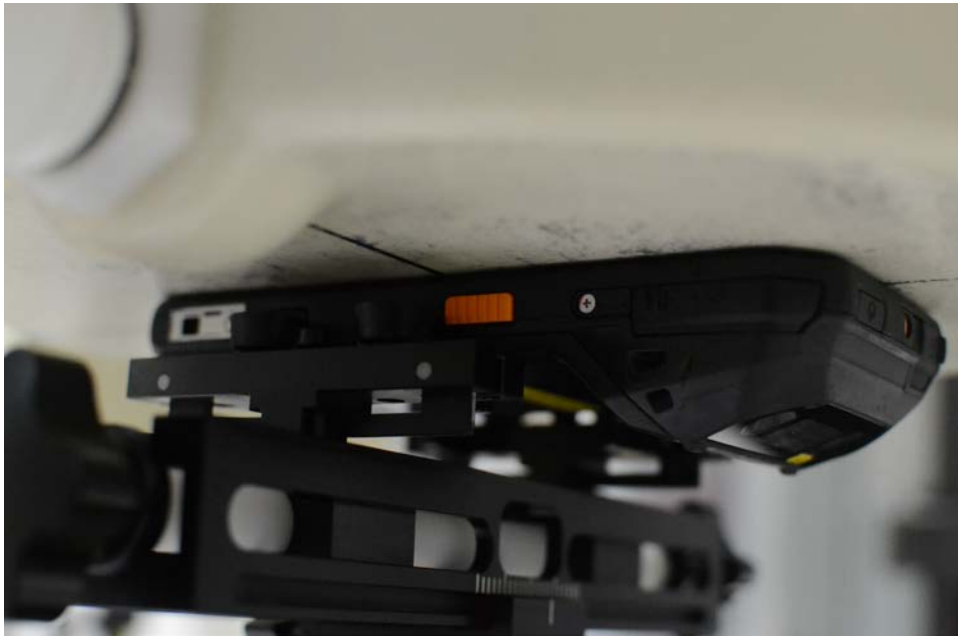
SAR Test Setup Photo 10: Front Side at 0.0 cm
