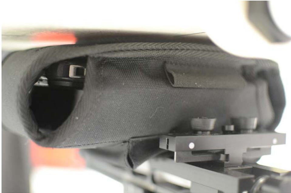
SAR Test Setup Photo 11: Front Side at 0.0 cm with Body Holster Accessory
