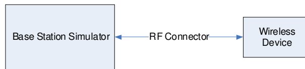
Figure 9-3 Power Measurement Setup
