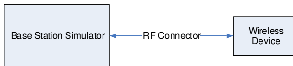
Figure 9-2 Power Measurement Setup
