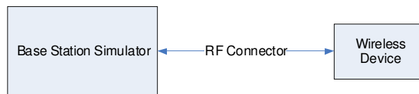
Figure 9-2 Power Measurement Setup
