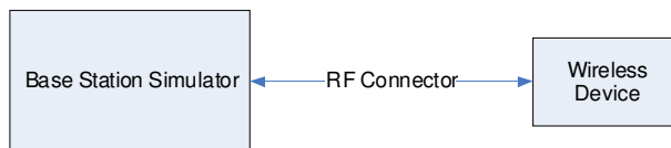
Figure 9-1 Power Measurement Setup
