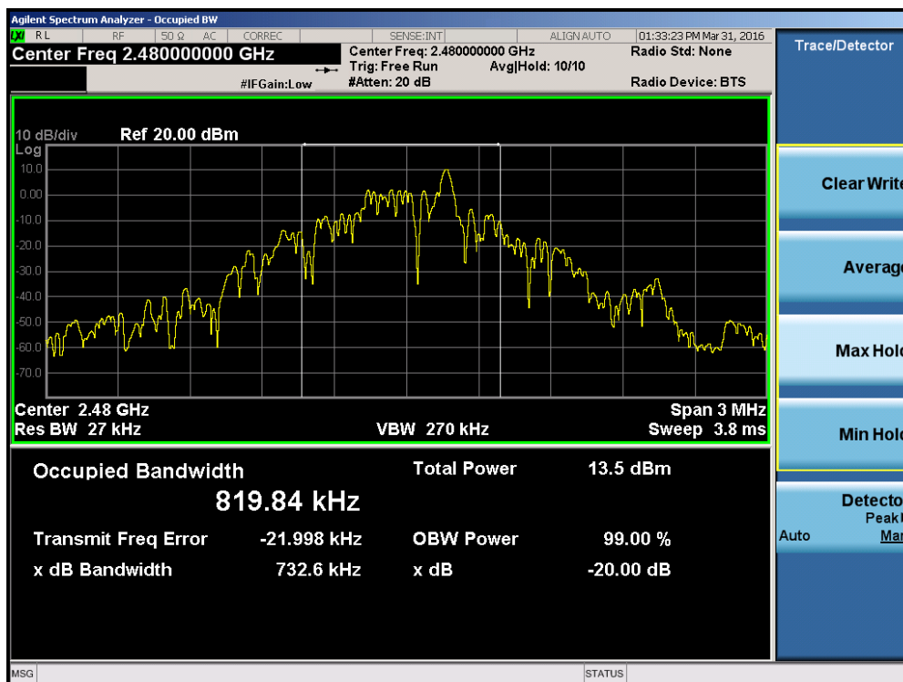
Plot 7-3. 20dB Bandwidth Plot (Bluetooth, 1Mbps – Ch. 78)
