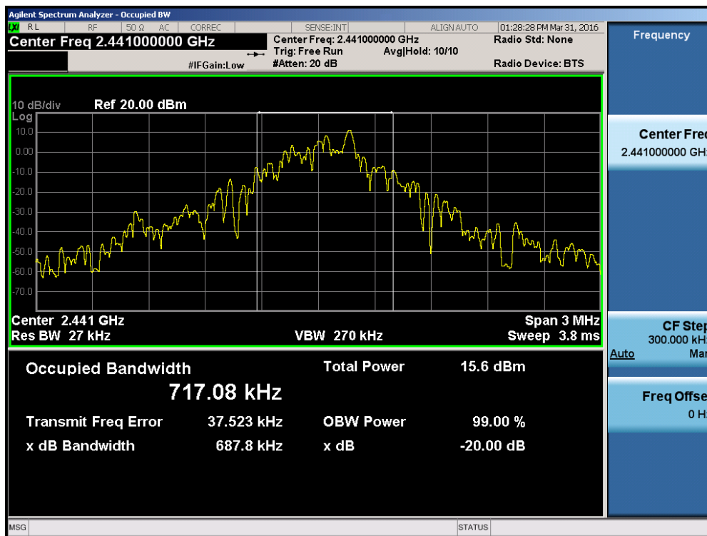
Plot 7-2. 20dB Bandwidth Plot (Bluetooth, 1Mbps – Ch. 39)
