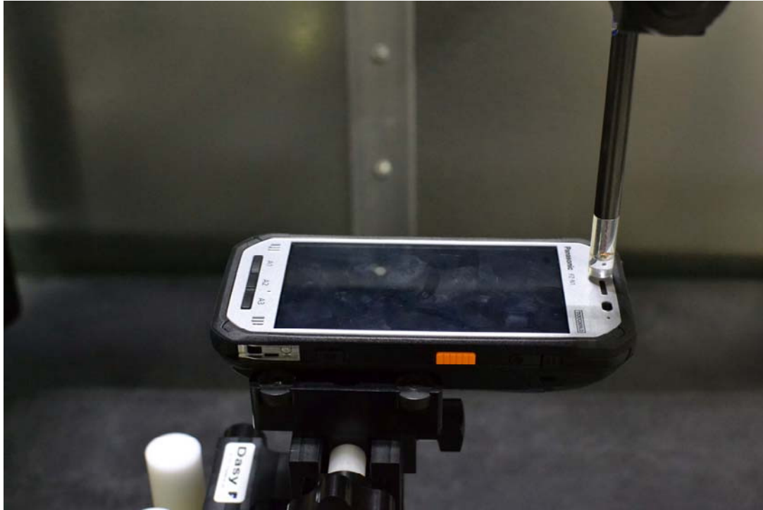
Figure 14-3 Test Setup for Wireless Device (L-Battery)
