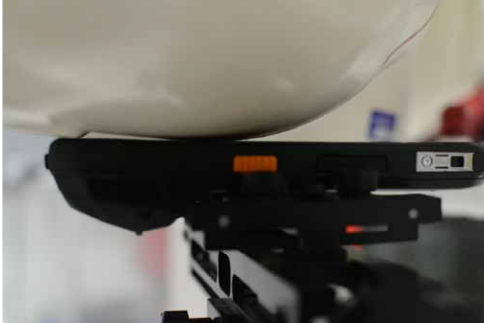
SAR Test Setup Photo 1 – Right Cheek with Standard Battery
