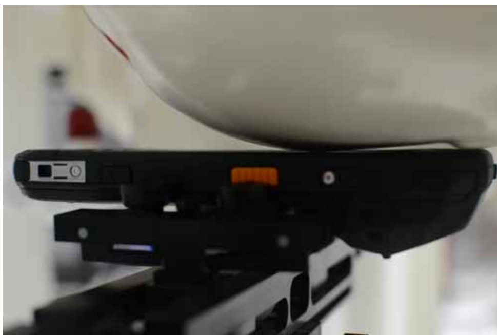
SAR Test Setup Photo 4 – Left Cheek with Standard Battery
