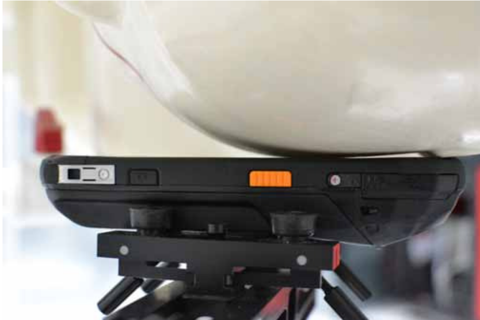
SAR Test Setup Photo 5 – Left Cheek with L-Battery
