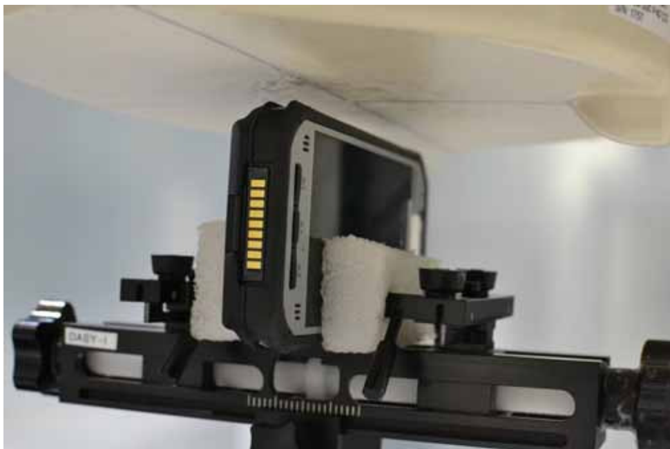
SAR Test Setup Photo 26 – Left Edge at 1.0 cm with L-Battery
