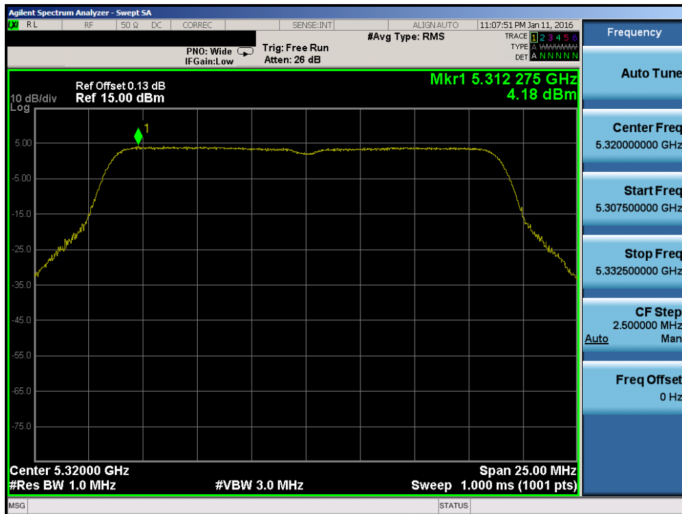
Plot 7-52. Power Spectral Density Plot (20MHz BW 802.11n (UNII Band 2A) – Ch. 64)
