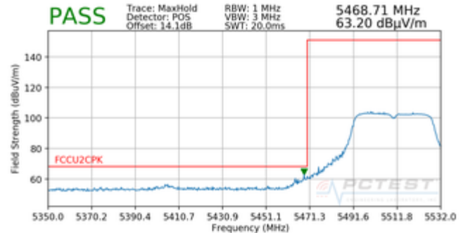
Plot 7-98. Radiated Lower Band Edge Plot (Peak – UNII Band 2C)
