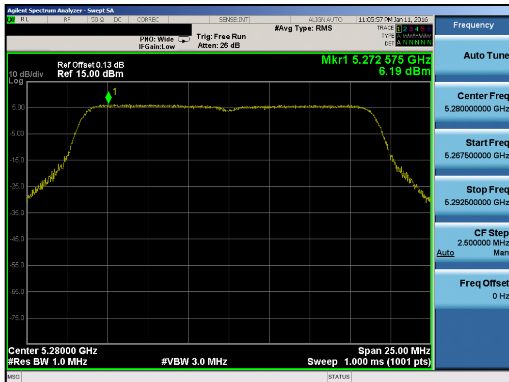
Plot 7-51. Power Spectral Density Plot (20MHz BW 802.11n (UNII Band 2A) – Ch. 56)
