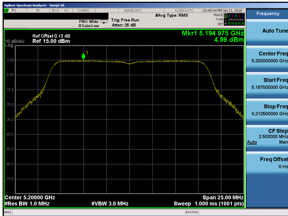
Plot 7-39. Power Spectral Density Plot (802.11a (UNII Band 1) – Ch. 40)
