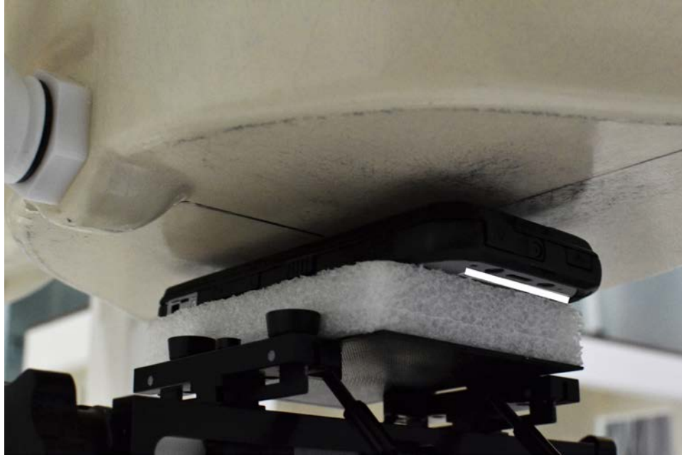
SAR Test Setup Photo 5: Back Side at 0.5 cm
