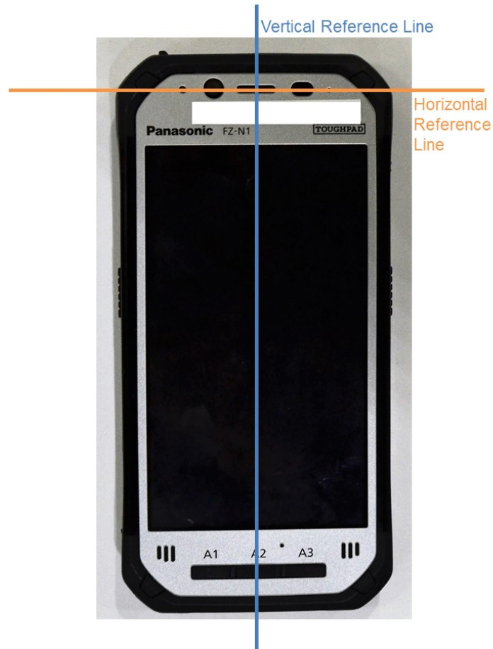
SAR Test Setup Photo 10: Horizontal and Vertical Reference Lines
