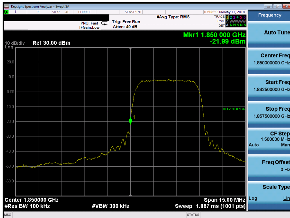
Plot 7-23. Band Edge Plot (PCS WCDMA Mode - Low Channel)
