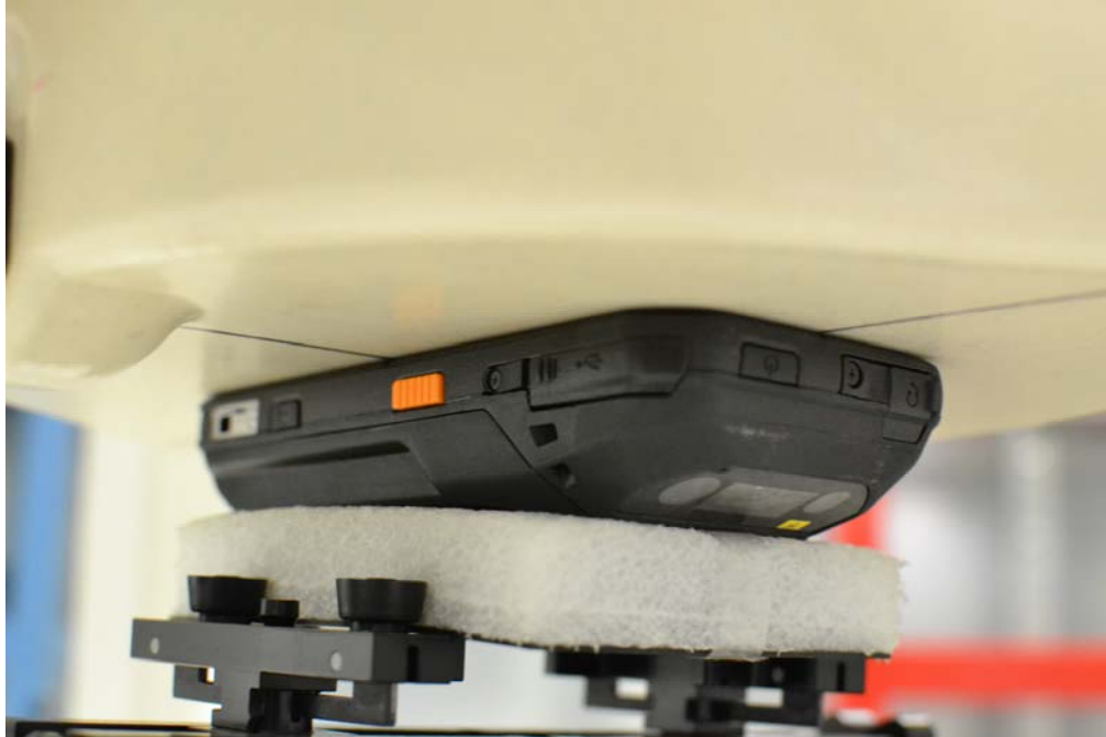
SAR Test Setup Photo 17 – Front Side at 0.0 cm with L-Battery
