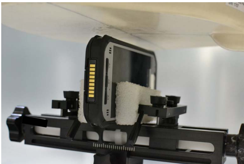
SAR Test Setup Photo 27 – Left Edge at 1.0 cm with Standard Battery
