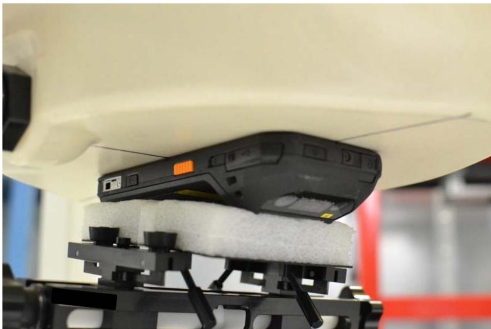
SAR Test Setup Photo 15 – Front Side at 0.0 cm with Standard Battery
