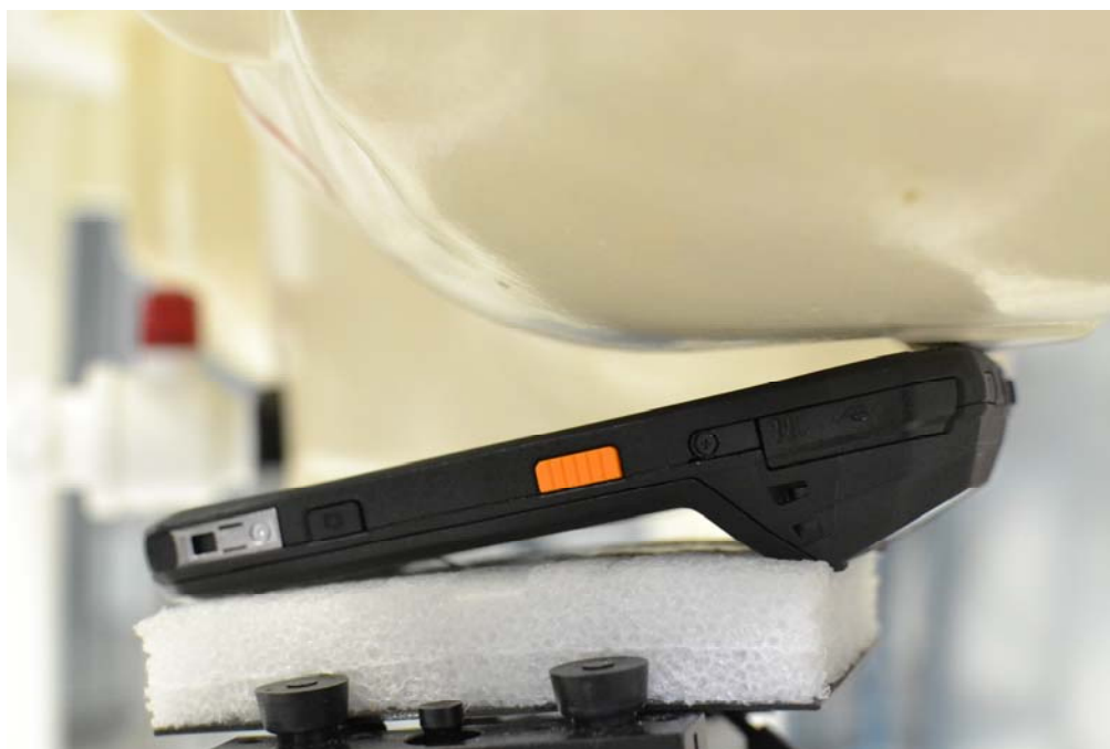
SAR Test Setup Photo 6 – Left Tilt with Standard Battery
