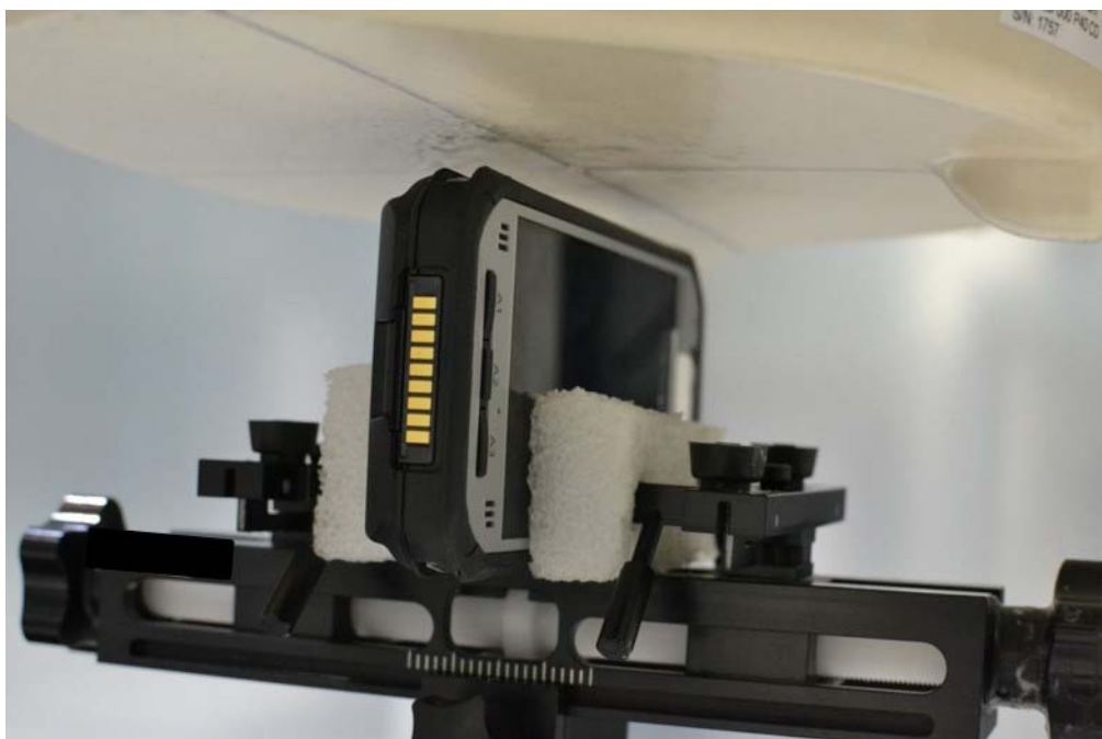
SAR Test Setup Photo 29 – Left Edge at 1.0 cm with L-Battery
