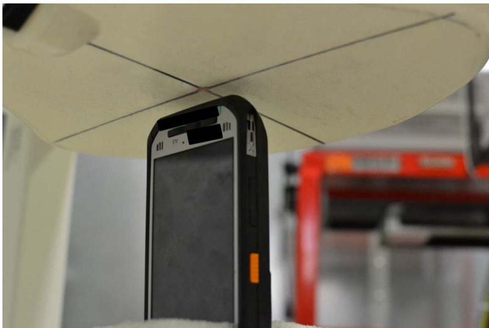
SAR Test Setup Photo 25 – Bottom Edge at 1.0 cm with L-Battery
