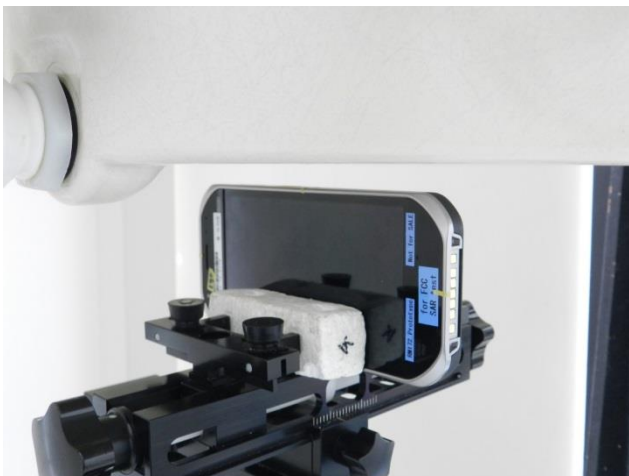
Right Side, Test Separation 10 mm
