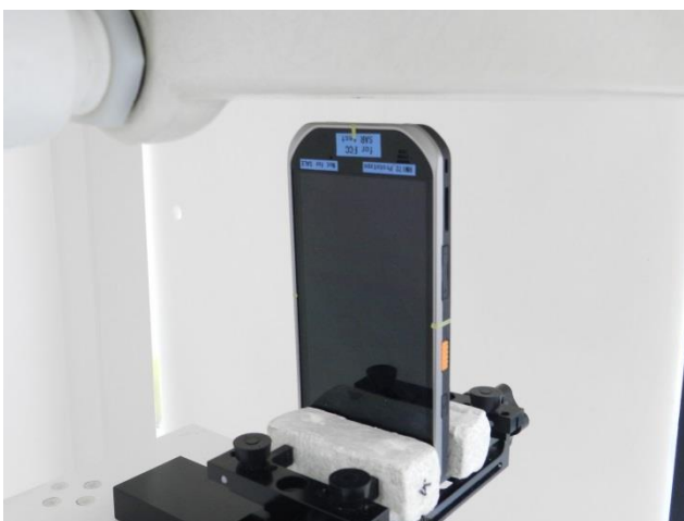
Bottom Side, Test Separation 10 mm
