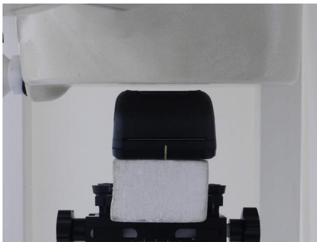
Back, Test Separation 5 mm
