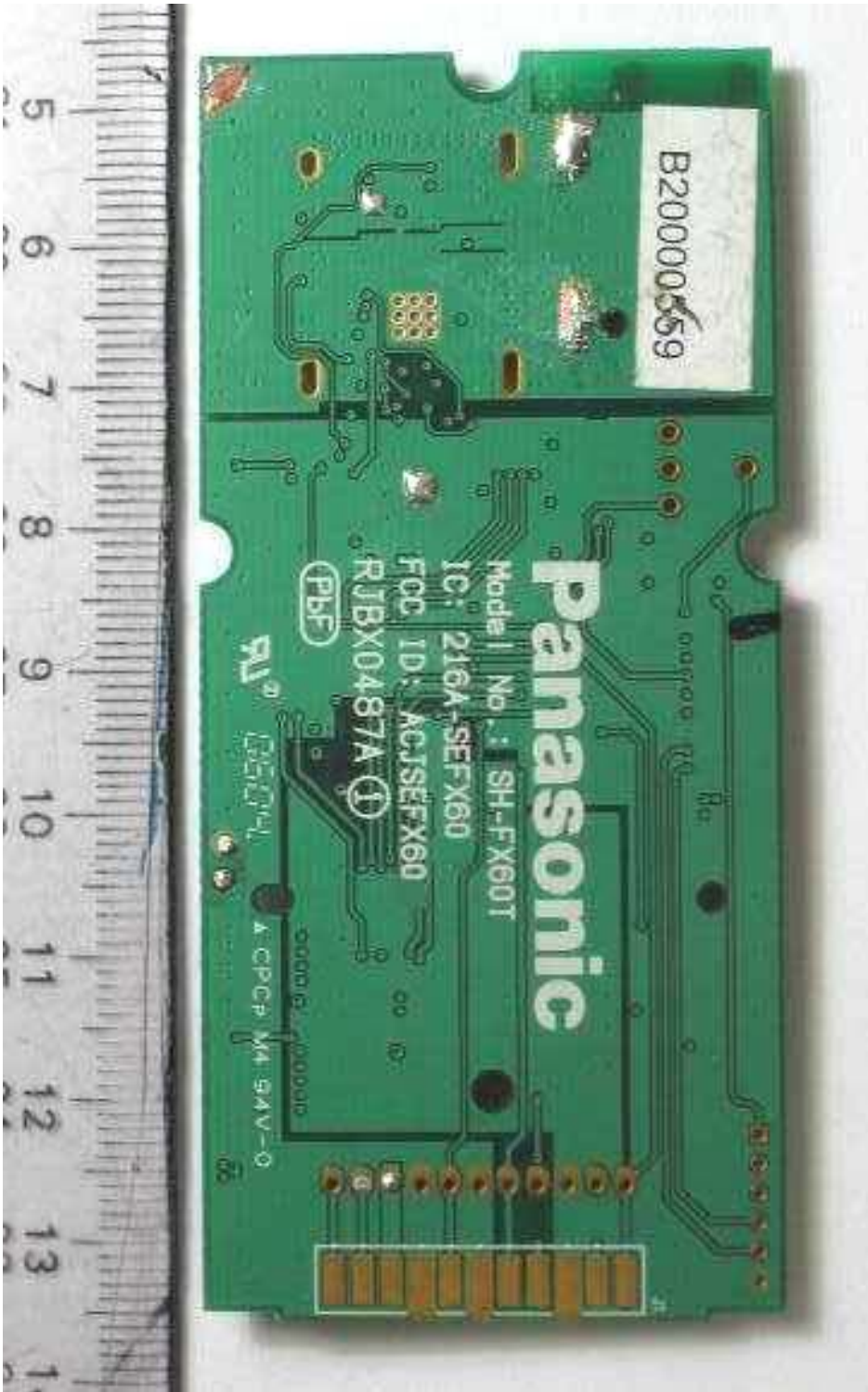
Rear View (RF Shield Removed)
