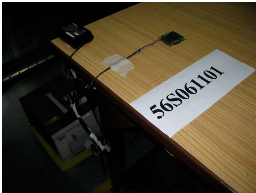
Conducted Emissions Test Setup (Rear View)
