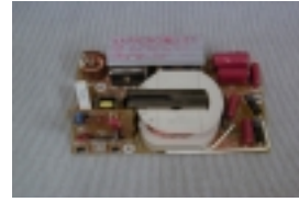
Exhibit 2-K, View of Inverter Power Supply
