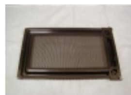
Exhibit 2-H, View of Door Construction illustrating integral choke
