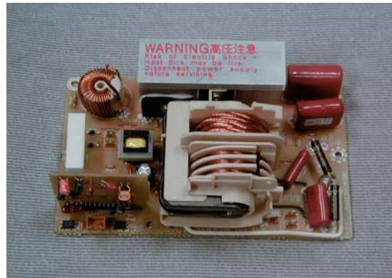
Exhibit 2-K View of Inverter Circuitry
