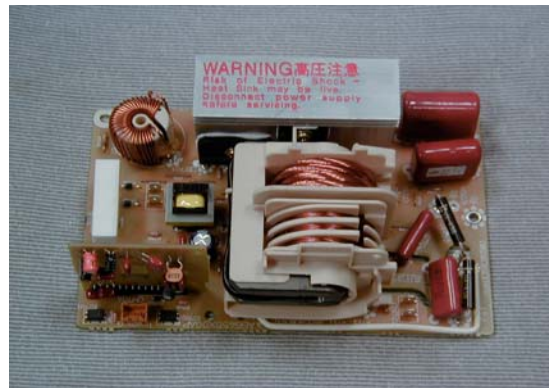
Exhibit 2-K View of Inverter Circuitry
