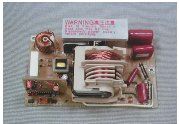
Exhibit 2-K View of Inverter Circuitry
