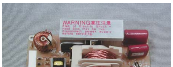
Exhibit 2-I View of Door Choke Constructio
