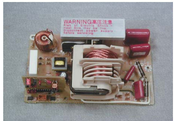
Exhibit 2-K View of Inverter Circuitry
