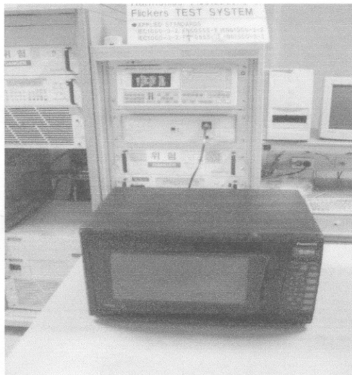
Fig.3 Test Setup for RF output power
