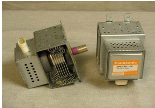
Exhibit 2-H View of Magnetron 2M236-M1
