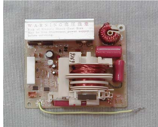
Exhibit 2-K View of Inverter Circuitry
