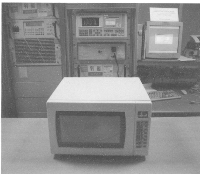
Fig.3 Test Setup for RF output power
