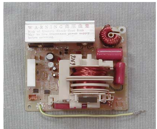
Exhibit 2-K View of Inverter (
