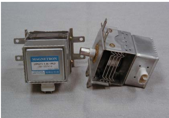
Exhibit 2-I View of Magnetron 2M211
