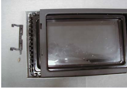
Exhibit 2-L View of Door Choke Construction
