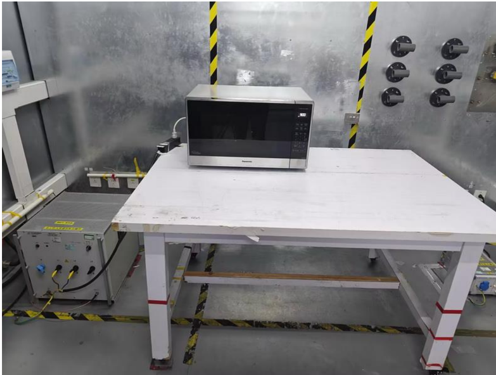
AC Power Line Conducted Emissions
