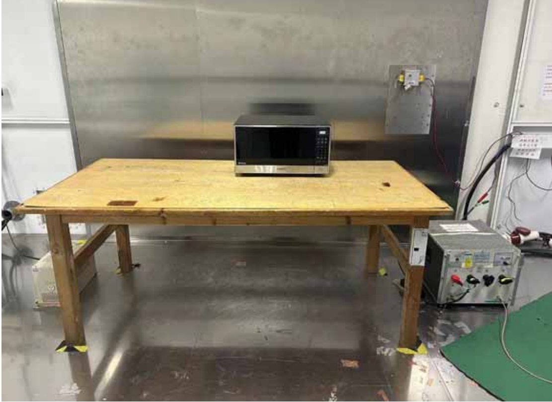
Front View of Conducted Measurement
