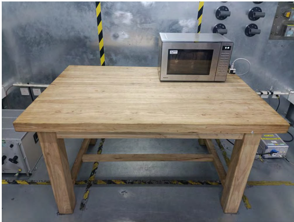
AC Power Line Conducted Emissions
