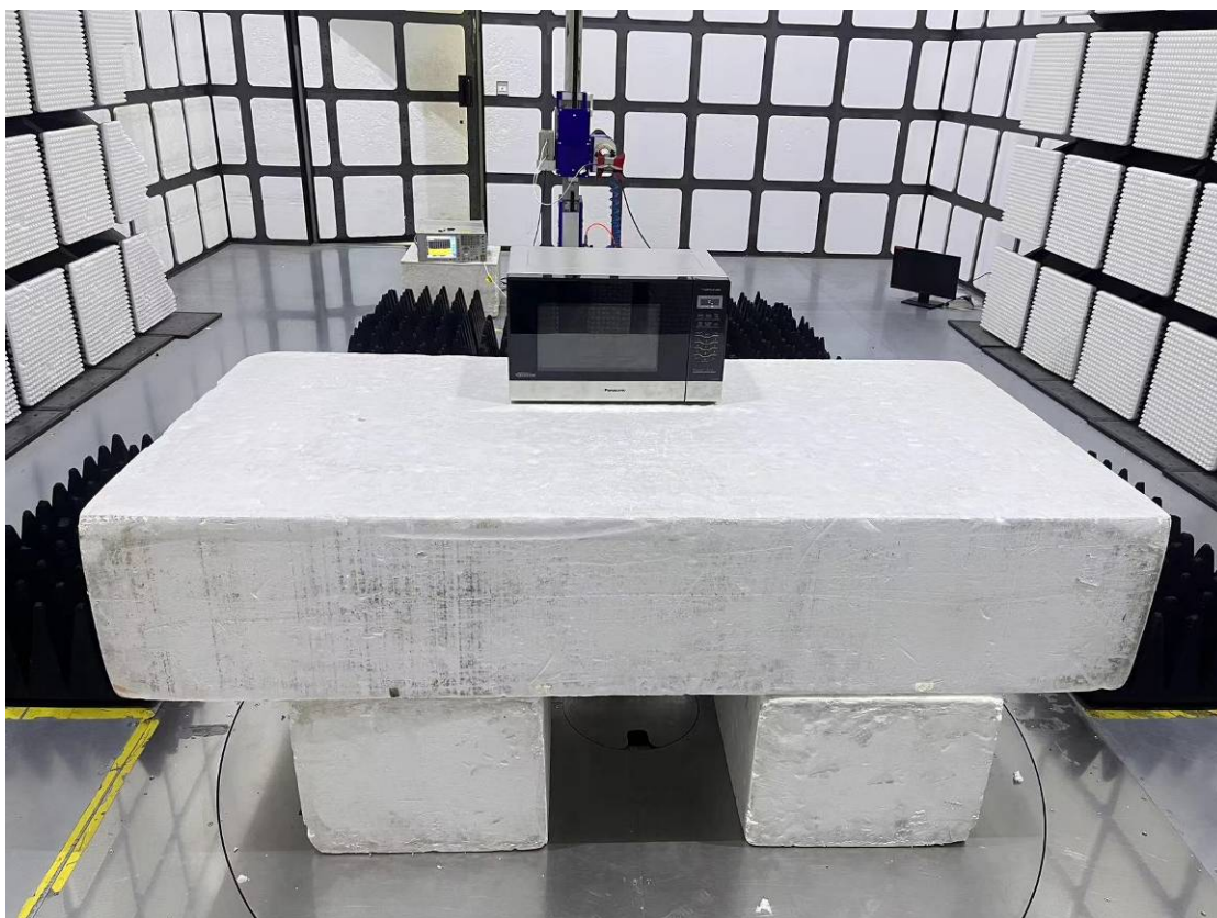
Front View of Radiated Measurement
