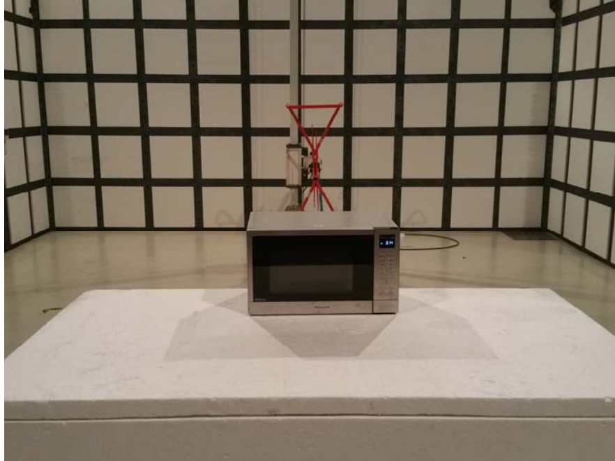
Radiated Disturbances Rear Side (Below 1GHz)
