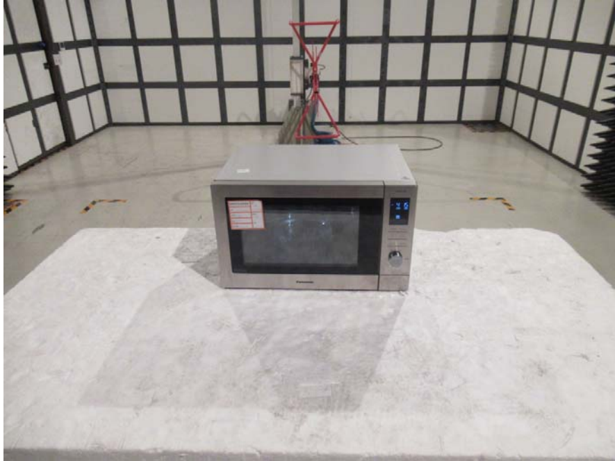
Radiated Disturbances Rear Side (Below 1GHz)
