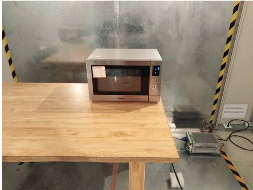
Conducted Emissions –Rear View
