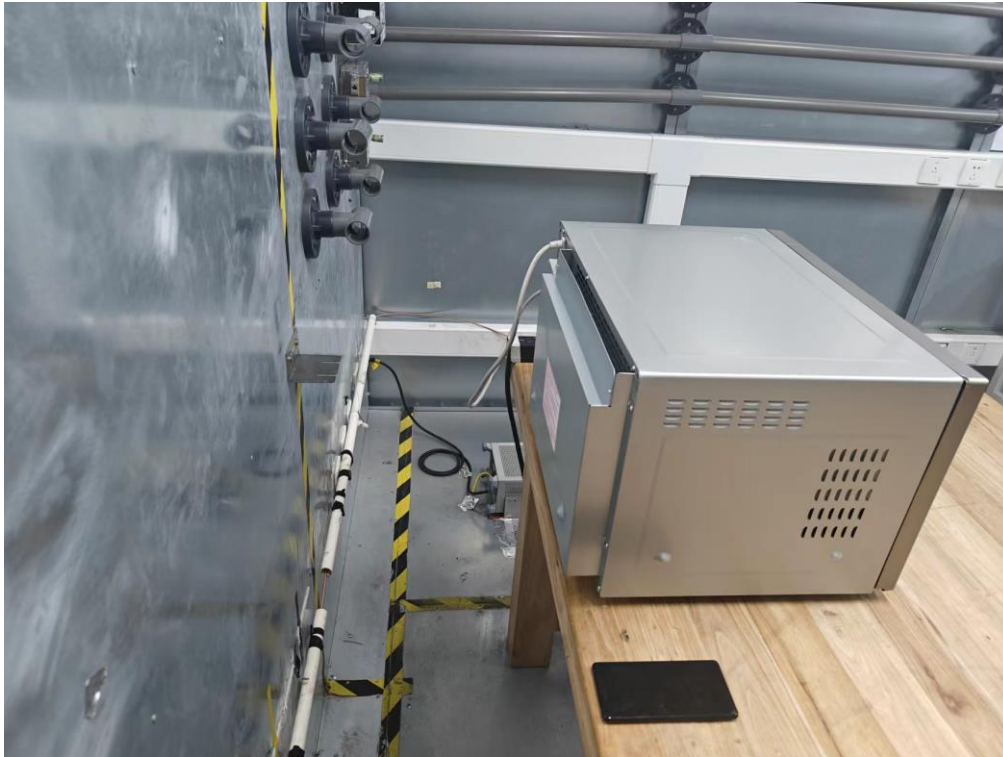
AC Power Line Conducted Emissions
